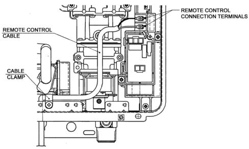
Fig. 8 Control Wiring Connections Inside Water Heater
